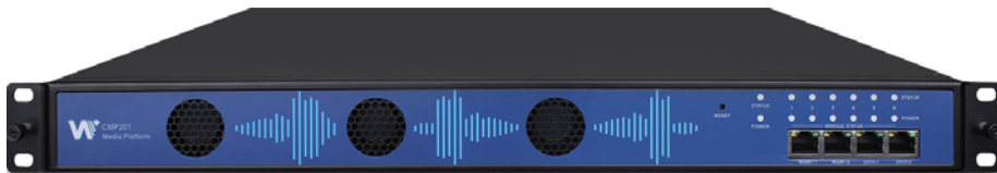
CMP201: 1RU chassis, single PSU, 6 swappable slots, 4 Gigabit network ports (2 NMS, 2 Data), 14 indicators
