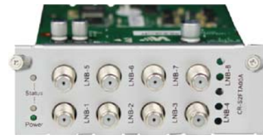
CR2-DVBS2FTA-01A DVB-S/S2/S2X FTA Receiver Module
