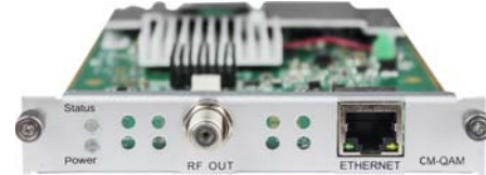
CM2-QAMA/B-R00: QAM Modulation Module
