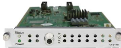
CM2-DTMB-R01/R01A: DTMB Modulation Module
