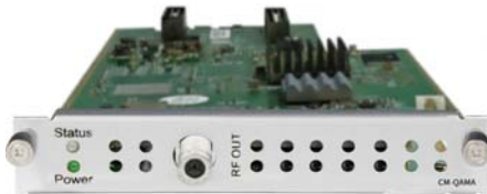
CM2-QAMA-R01/R01A: QAMA Modulation Module
